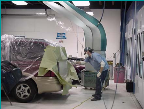
Duster 3000 Downdraft in an autobody shop
