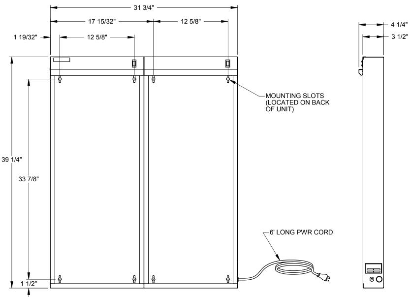
Electrical Requirements: 120VAC, 60 Hertz, Single Phase Power Rating: 2.4A
