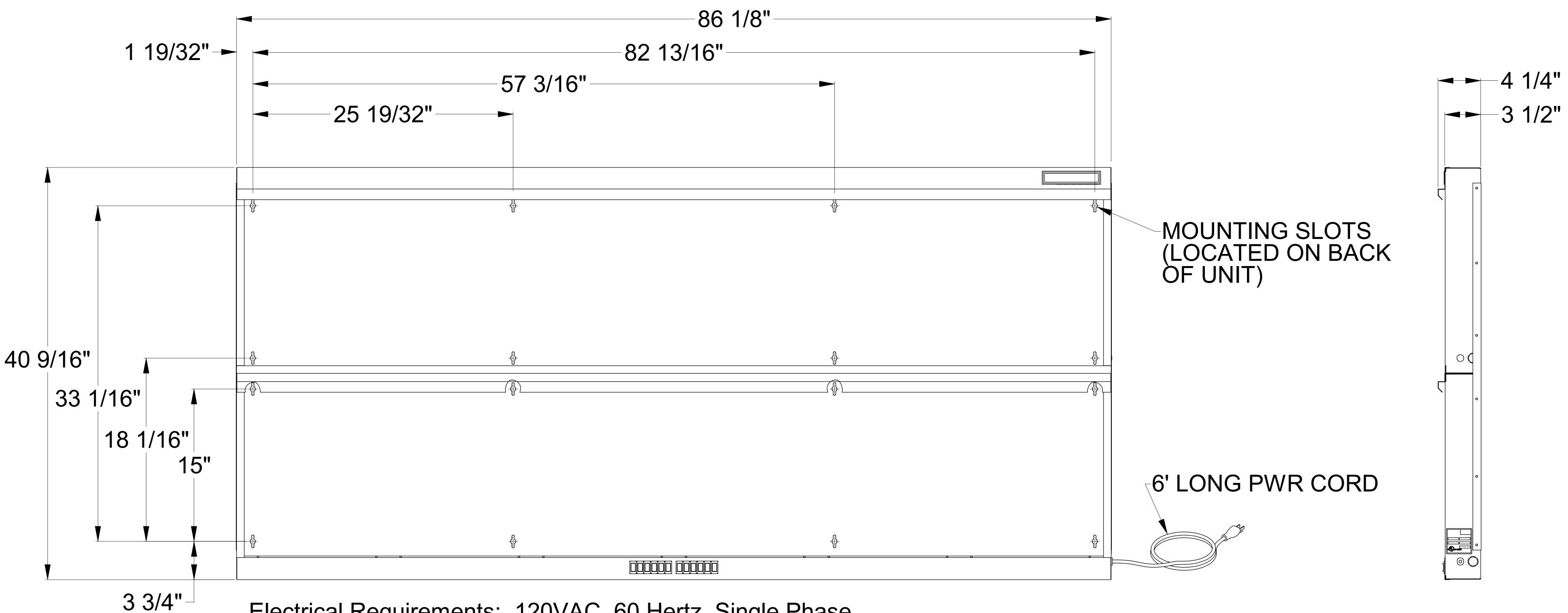
Electrical Requirements: 120VAC, 60 Hertz, Single Phase Power Rating: 14.4A
