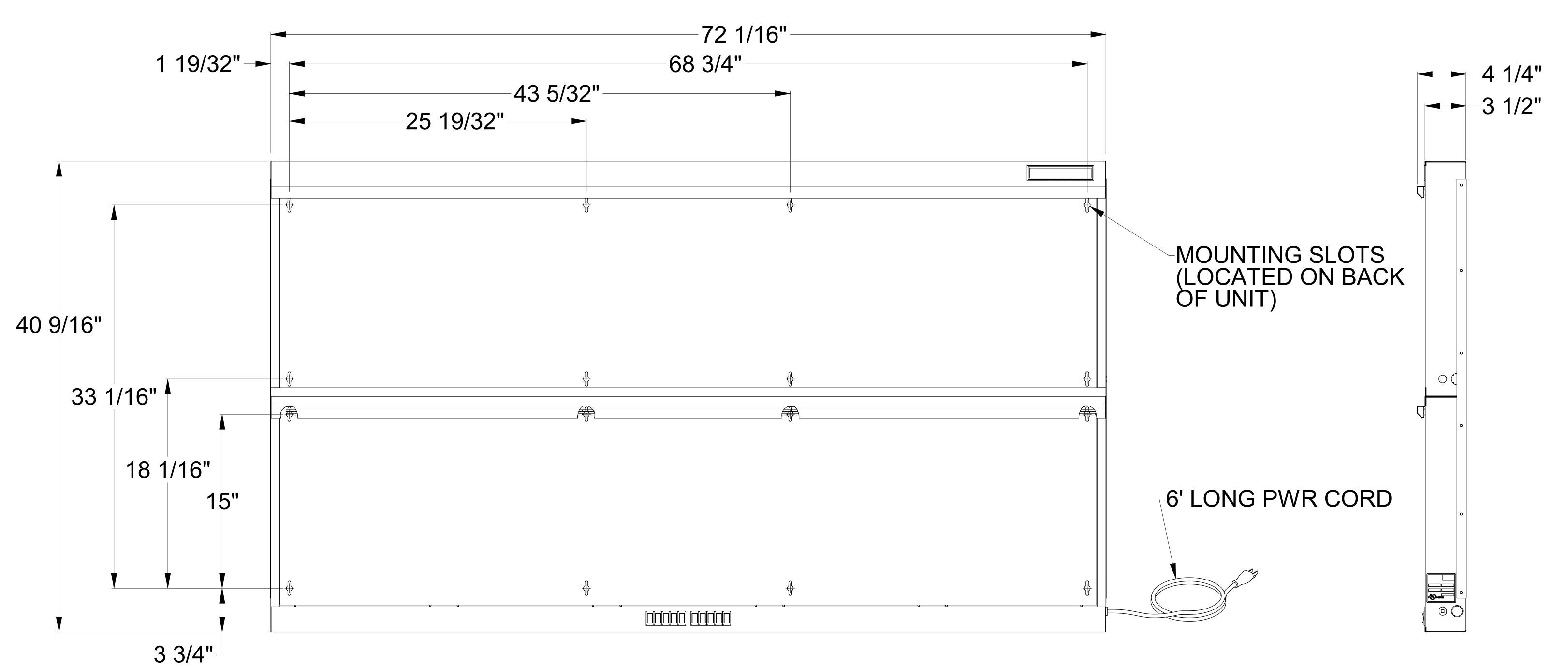
Electrical Requirements: 120VAC, 60 Hertz, Single Phase Power Rating: 12A
