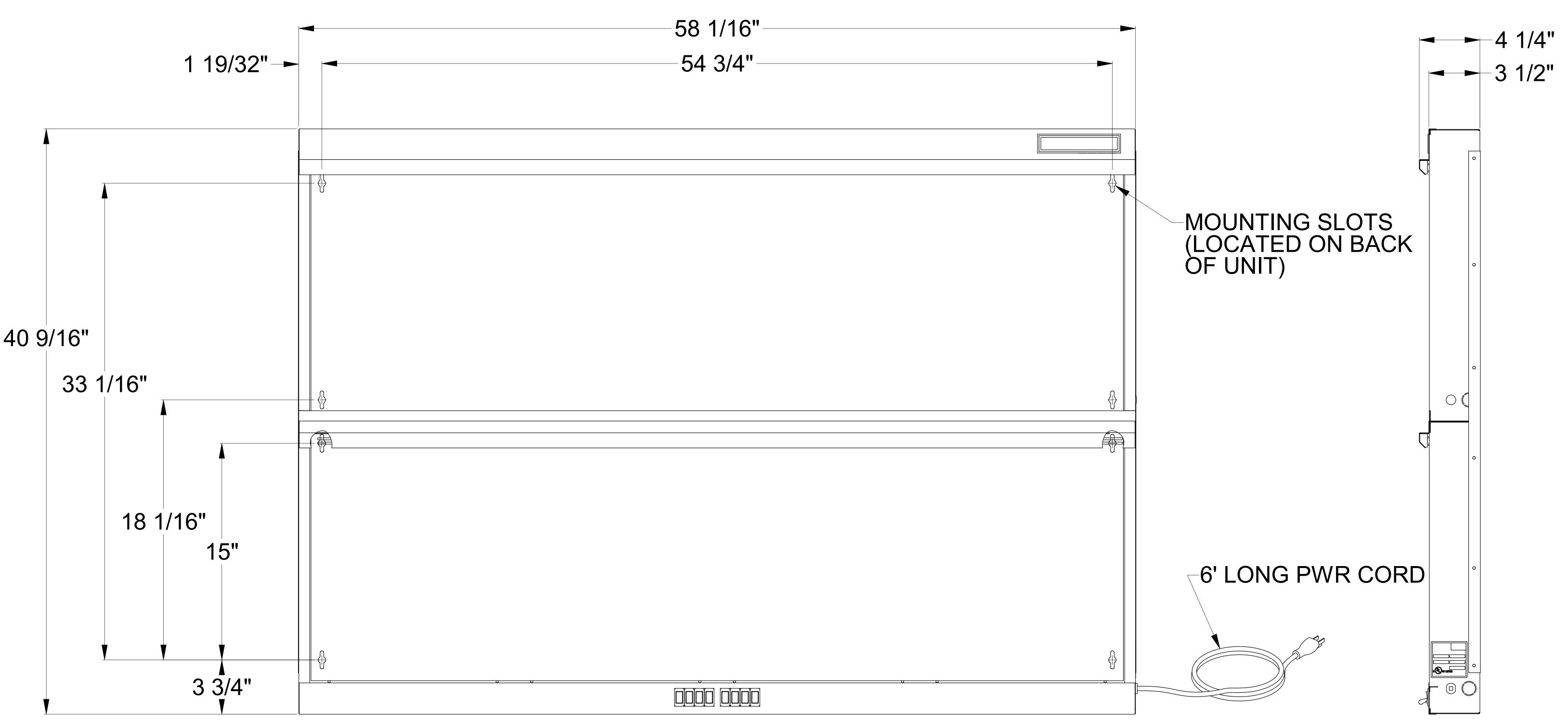
Electrical Requirements: 120VAC, 60 Hertz, Single Phase Power Rating: 9.6A
