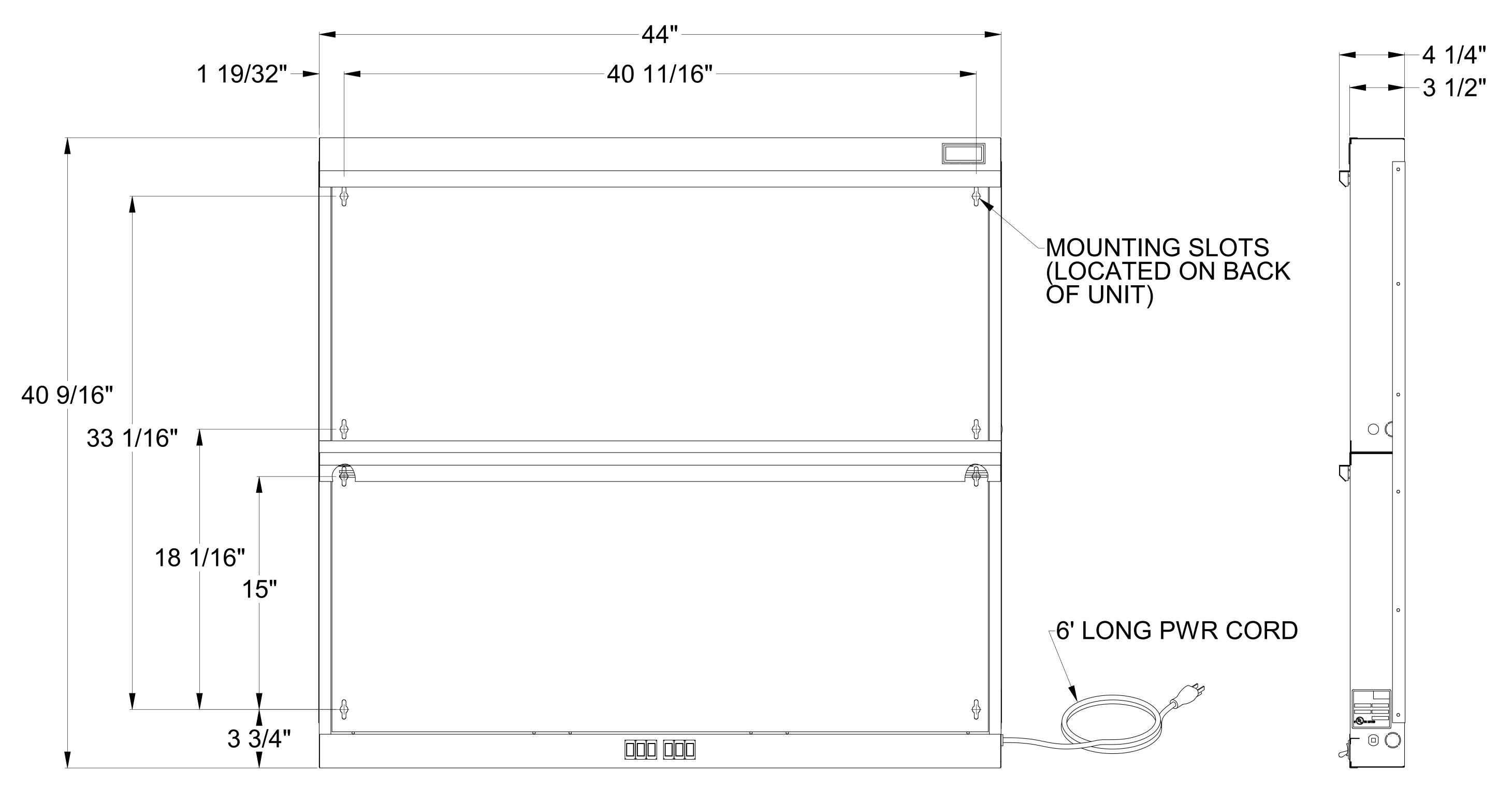
Electrical Requirements: 120VAC, 60 Hertz, Single Phase Power Rating: 7.2A
