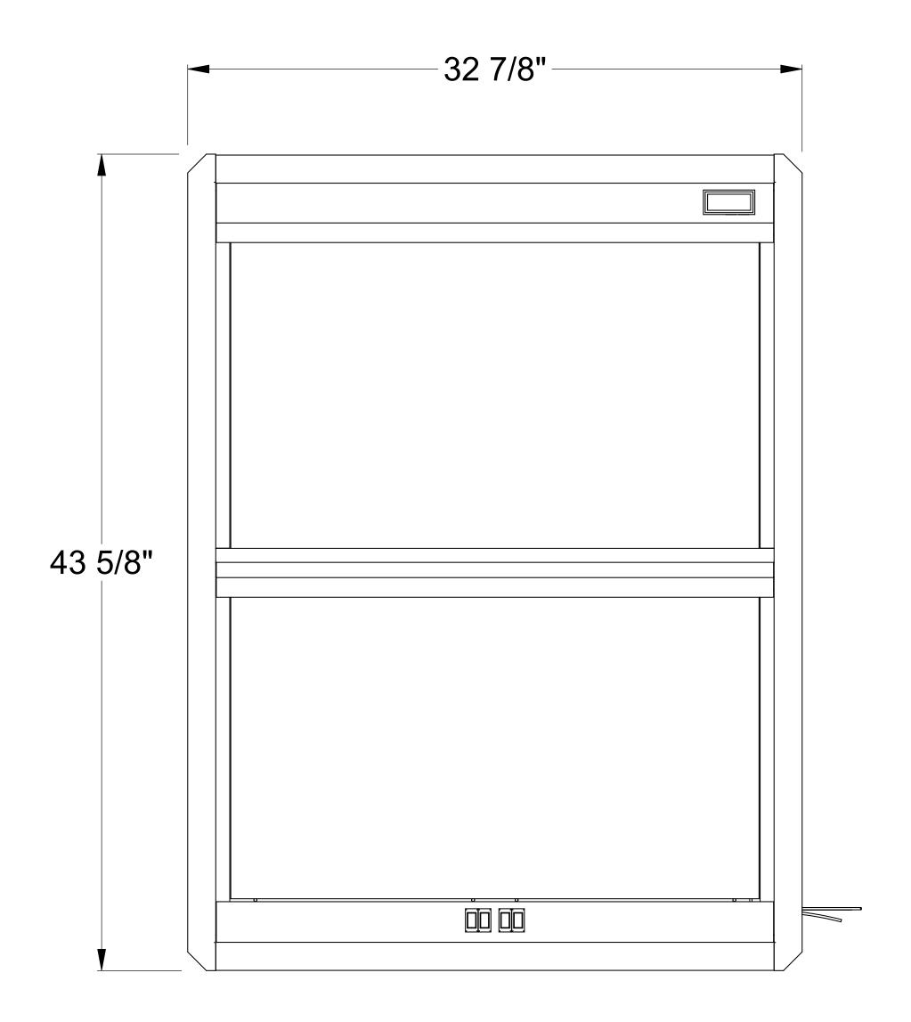
Electrical Requirements: 120VAC, 60 Hertz, Single Phase Power Rating: 4.8A Rough Opening Dimensions: 41 1/4" x 30 5/8" UL/CUL Approved
