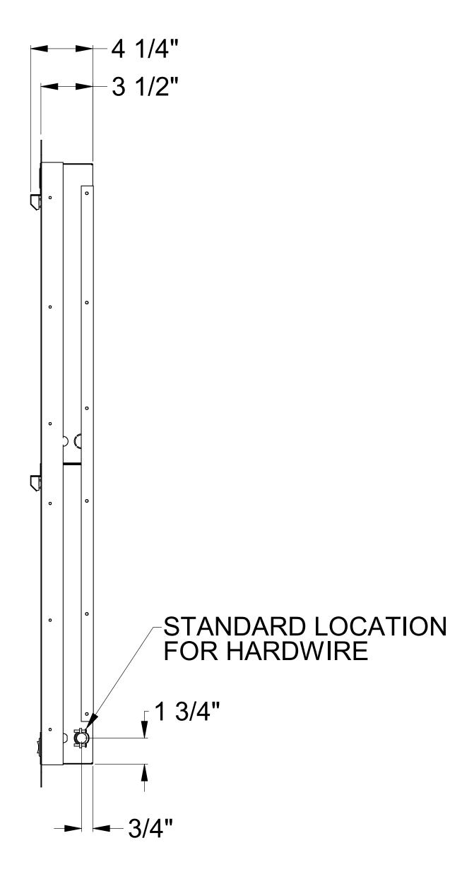
Electrical Requirements: 120VAC, 60 Hertz, Single Phase Power Rating: 2.4A Rough Opening Dimensions: 41 1/4" x 16 5/8"
