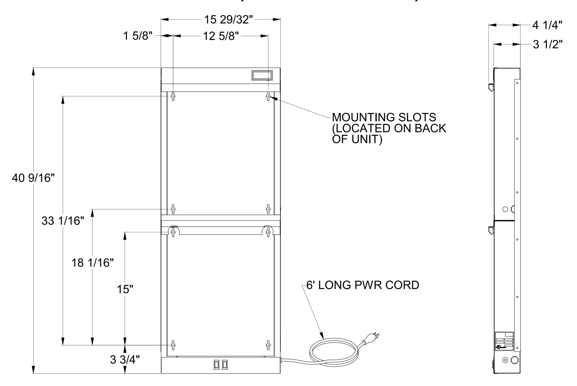
Electrical Requirements: 120VAC, 60 Hertz, Single Phase Power Rating: 2.4A
