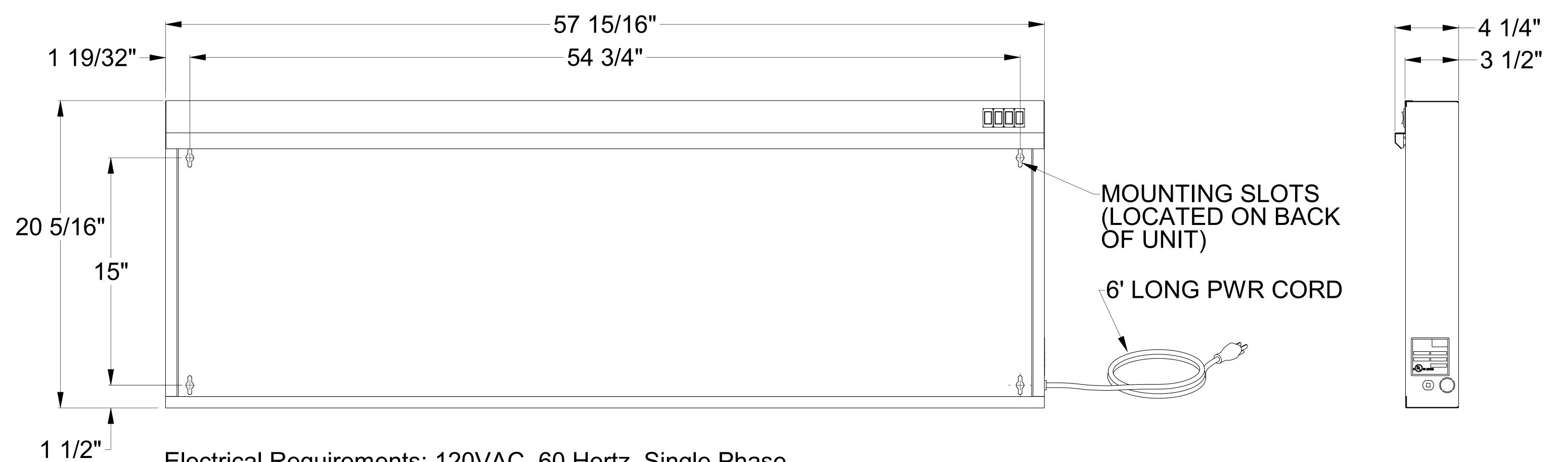
Electrical Requirements: 120VAC, 60 Hertz, Single Phase Power Rating: 4.8A
