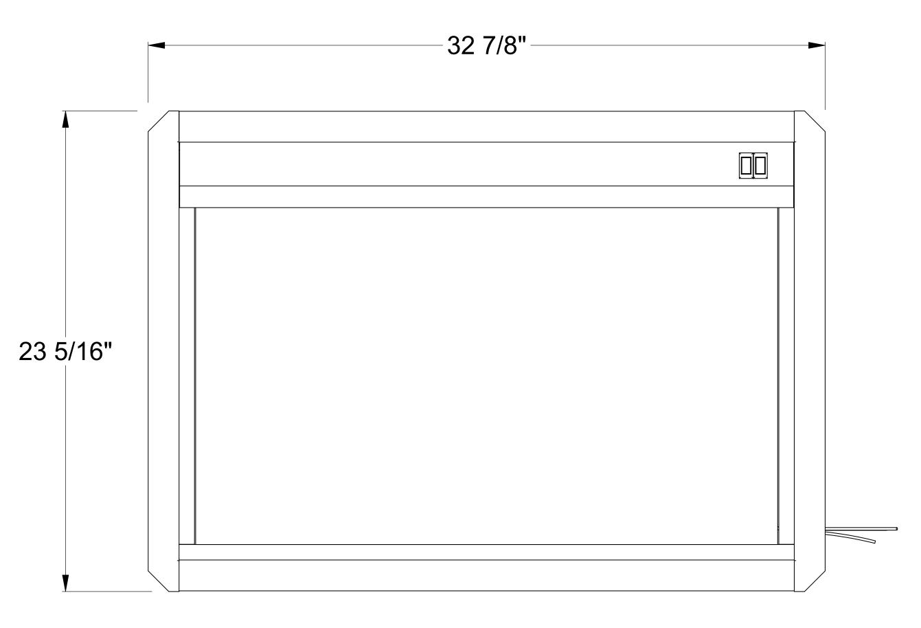
Electrical Requirements: 120VAC, 60 Hertz, Single Phase Power Rating: 2.4A Rough Opening Dimensions: 21" x 30 5/8"
