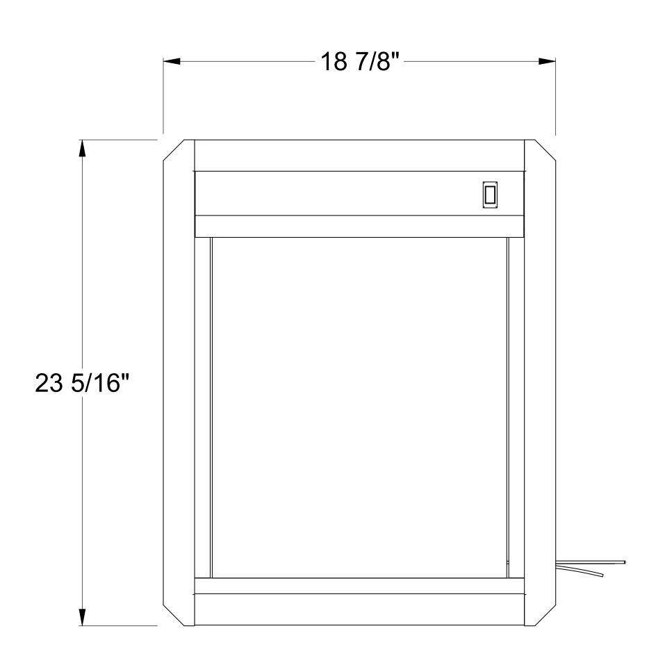
Electrical Requirements: 120VAC, 60 Hertz, Single Phase Power Rating: 1.2A Rough Opening Dimensions: 21" x 16 5/8"
