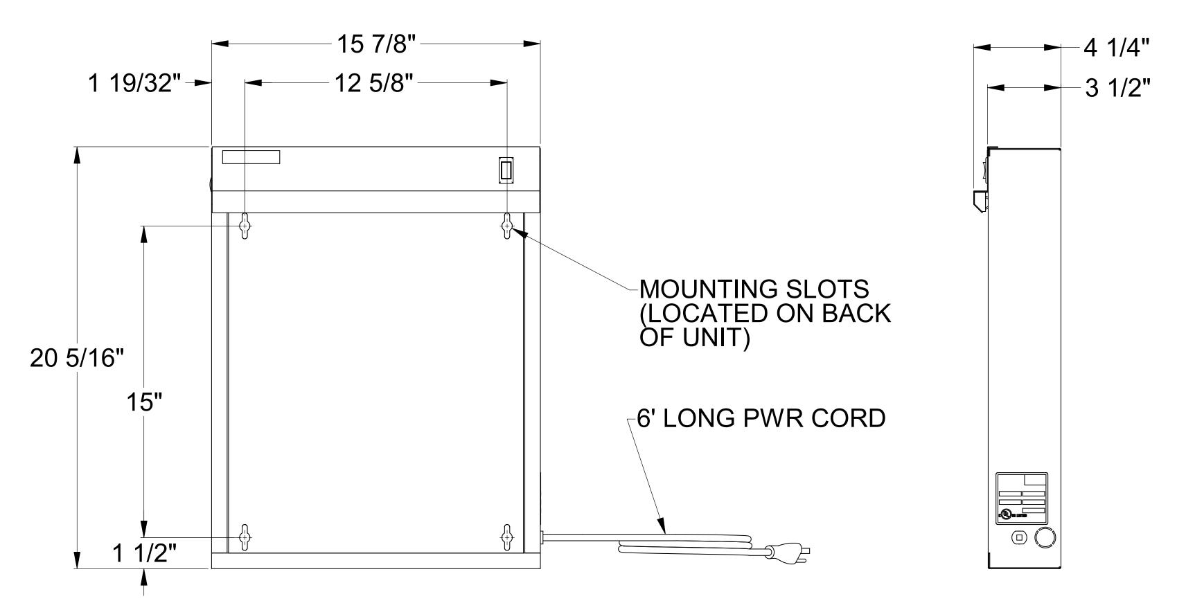
Electrical Requirements: 120VAC, 60 Hertz, Single Phase Power Rating: 1.2A
