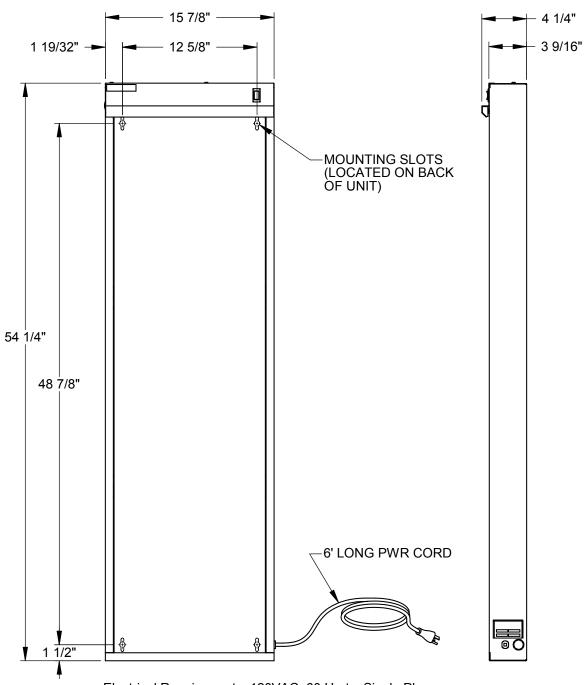
Electrical Requirements: 120VAC, 60 Hertz, Single Phase Power Rating: 1.2A
