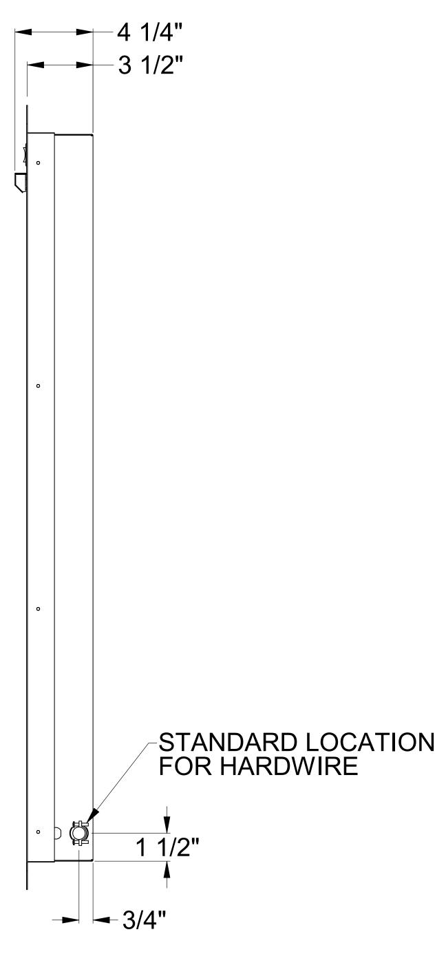
Electrical Requirements: 120VAC, 60 Hertz, Single Phase Power Rating: 1.4A Rough Opening Dimensions: 39 7/8" x 16 5/8"
