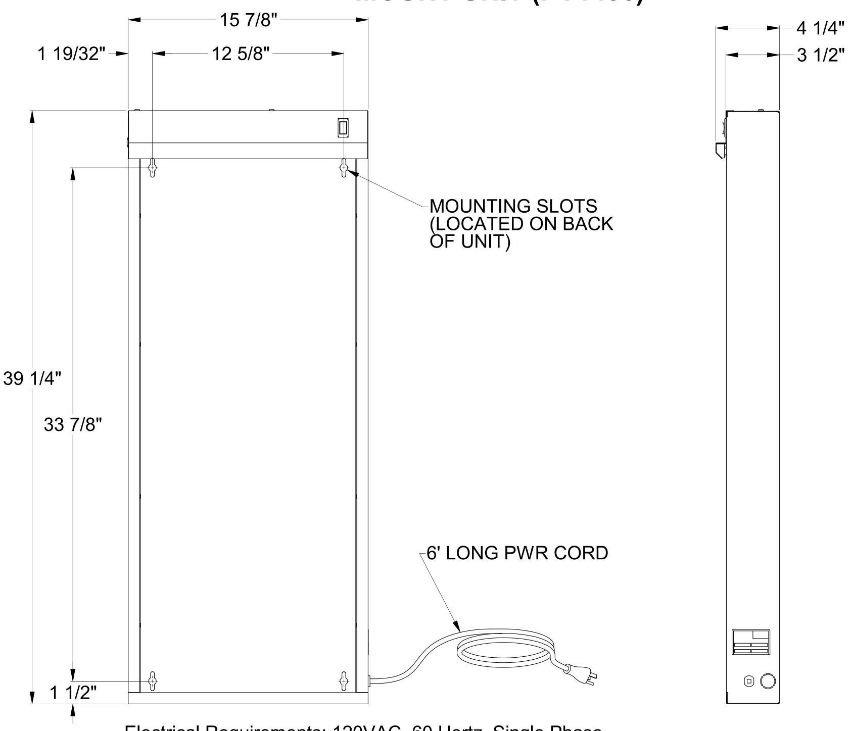
Electrical Requirements: 120VAC, 60 Hertz, Single Phase Power Rating: 1.4A
