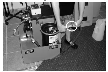
7. Move the #2 cartridge to the #1 position. Attach fitting from bottom of cartridge to fitting from machine.
