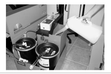
2. Allow all the water to pump through the Cartridges, perhaps overnight.(2 gallons of water will take 1-1/4 hours)
