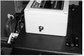
4. Using the quick disconnect fittings on the cartridges, disconnect cartridge #1 from the machine and from cartridge #2.
