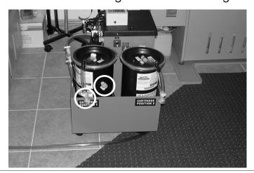
12.. Turn machine power on. Pour 4 gallons of water in the holding tank.
