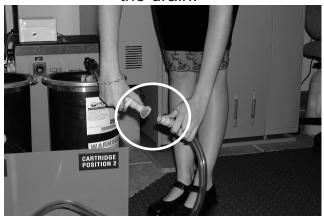
8. Remove the new cartridge from the shipping container. **DO NOT THROW AWAY THE BOX OR PACKING MATERIAL**.
