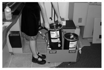
6. Disconnect #2 cartridge from the hose leading to the drain.
